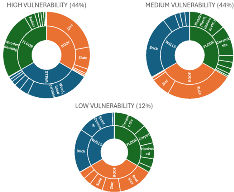
Figure 3: Results of the latent-class-analysis model estimated on census data: distribution of seismic vulnerability classes and of building materials within each class ( N=929,647 ). Notes: The percentages next to each class label represent the proportion of homes in that class in the population of households with at least one school-aged child in the 2002 census.
