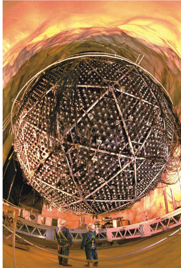
Sudbury Neutrino Observatory in Canada, 2 km underground. The 12 meter diameter tank contains 1,000 tons of heavy water.
