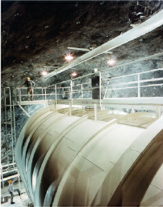
Homestake Neutrino Detector in South Dakota, 1.5 km underground. Neutrino detectors are placed underground to shield them from other unwanted interaction with other cosmic ray particles.
