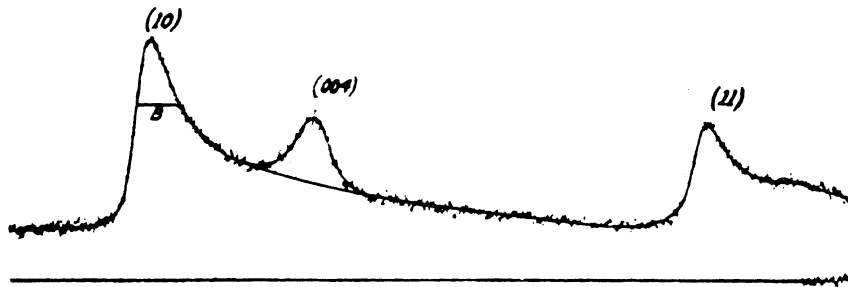
FIG. 4. Microphotometer record of the diffraction pattern of a heat treated carbon black, showing two-dimensional lattice reflections. Radiation \text{Cu } K\alpha = 1.539 monochromated by reflection from rocksalt.
