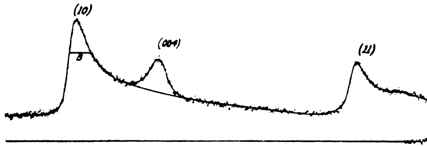
FIG. 4. Microphotometer record of the diffract pattern of a heat treated carbon black, showing three-dimensional lattice reflections. Radiation \text{Cu } K\alpha = 1.539 \text{ \AA} monochromated by reflection from rocksalt.
