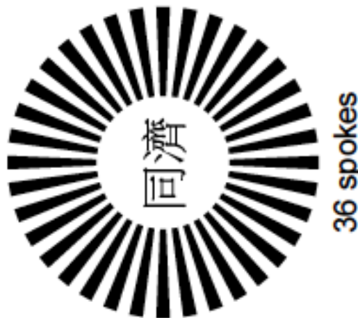
Figure 46 Schematic diagram for Siemens-star Test pattern with 36 spokes; sample is made of Tungsten, 1.5 microns thick, for hard X-ray measurements. Fabricated by zoneplates.com, Courtesy Dr. Graeme Morrison, University College London, UK
