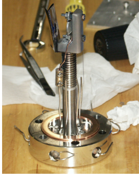
Figure 4.10: Side view of sample mount, showing shield (folded), the back of the heater, the ceramic block, the thermocouple wires, and wires to power the heater.
