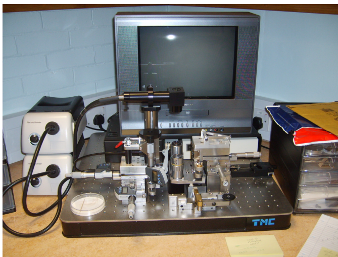
Figure 2. 8: Pre-alignment optical microscope system of the NanoXCT from Xradia.
