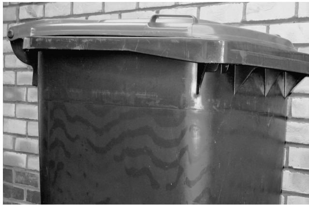
Figure 2. Wheeled bin showing the ‘tiger stripes’ characteristic of an unstable fountain flow during manufacture.
