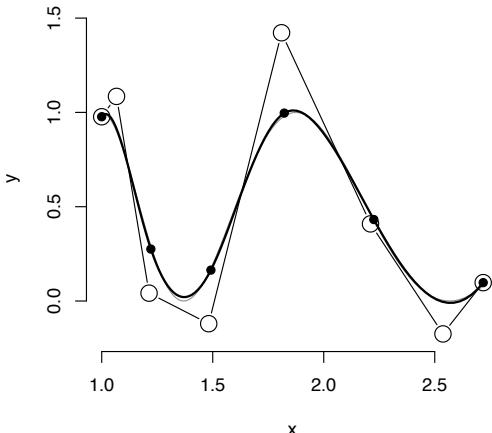
**Figure 8.2:** Cubic B-spline approximation to the 2-D parametric function  $(t^4 \cos^2 5t)$  over the interval  $[0, 1]$ , using four internal knots. The thick black line is the spline curve, filled circles represent knot points and open circles control points. The true function is shown in grey, but it is barely visible because the B-spline approximates it very closely.
