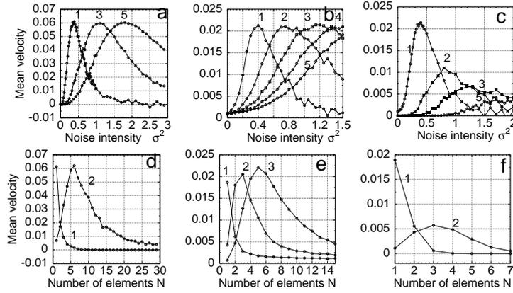
Fig. 3 – a, b, c: mean velocity *vs.* noise intensity for  $N = 1, 2, \dots, 5$ ,  $A = 1.15$ ,  $\omega = 0.1$ . d, e, f: mean velocity *vs.*  $N$  for different temperatures: d)  $\sigma^2 = 0.3$  (1), 2 (2); e)  $\sigma^2 = 0.3$  (1), 1 (2), and 2 (3); f)  $\sigma^2 = 0.5$  (1) and 1.5 (2). a, d: periodic force, b, e: colored noise, c, f: without global fluctuations.
