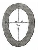
**Figure 1**: Conventional and egg-shaped sewers *Source*: PP, 1847/48, xxxii, 34
