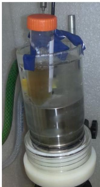
Figure 5.6: Suspension of graphene oxide in aniline
