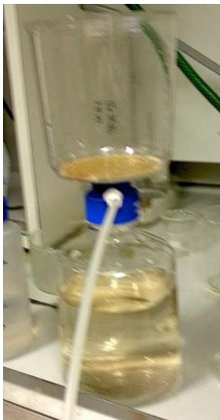
Figure 4.9: Buchner flask and funnel setup
