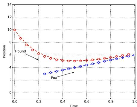
Figure 5: A pursuit curve. Arrows indicate velocity directions.
