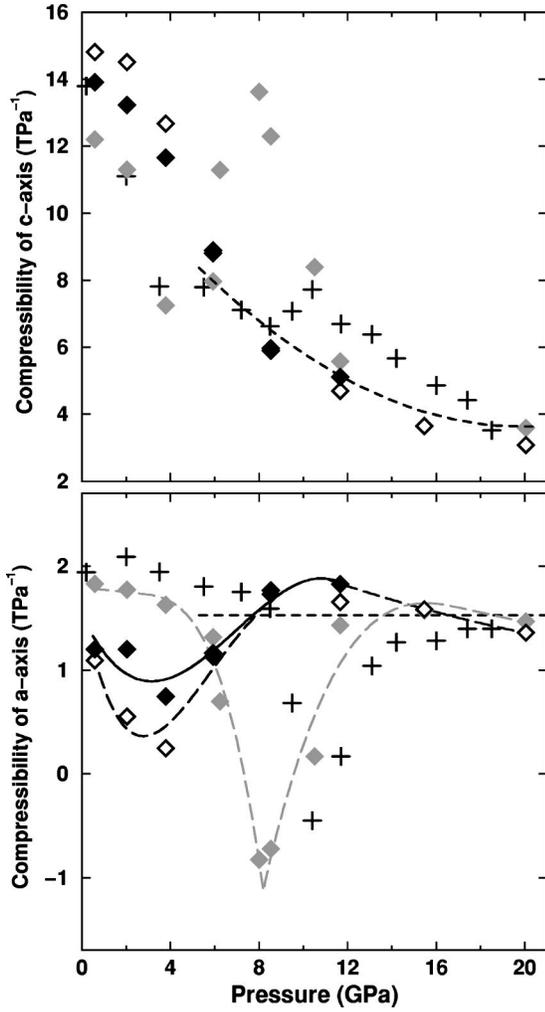
FIG. 4. Compressibility of the two axes  $k_a$  and  $k_c$  for our results ( $k$ -point sampling  $24 \times 24 \times 24$  with grey diamonds, for  $32 \times 32 \times 32$  and  $48 \times 48 \times 48$  we use a fit to the results in the long dashed and solid line, respectively) and static experiments using a methanol-ethanol-water mixture (pluses, Ref. 7) and helium (average in dashed line, Ref. 12) as a pressure pressure medium.
