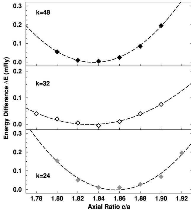
FIG. 2. Relative energies as a function of the axial ratio  $c/a$  for  $V=97.5$  Bohr<sup>3</sup>. The lower, middle, and upper panel shows results for  $24 \times 24 \times 24$ ,  $32 \times 32 \times 32$ , and  $48 \times 48 \times 48$   $k$  points, respectively. The lines show quadratic fits in  $c/a$  to the results.
