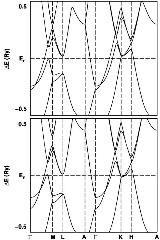
FIG. 5. Band structure for zinc along high-symmetry directions in the first Brillouin zone around the Fermi energy. The upper panel shows the band structure at zero pressure ( $V=102.5 \text{ Bohr}^3$ ), the lower panel at  $V=95 \text{ Bohr}^3$  at their equilibrium  $c/a$  (1.91 and 1.79, respectively).
