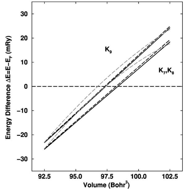
FIG. 6. Energy differences of the bands to the Fermi energy at the high-symmetry point  $K$  on the first Brillouin-zone boundary as a function of unit-cell volume. Gray dashed, dashed, and solid lines are results for  $k$ -point sampling of  $24 \times 24 \times 24$ ,  $32 \times 32 \times 32$ , and  $48 \times 48 \times 48$ , respectively.
