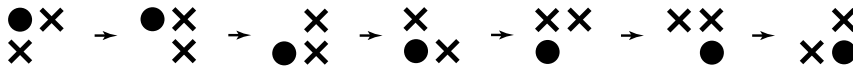
Figure 1. Schematic of the individual steps of the six jump cycle of solid-state diffusion. ● and × denote two different chemical species, with ● ultimately exchanging positions with a vacancy. This sequence of jumps is energetically more favorable than a single diagonal jump of ● into the vacancy.
