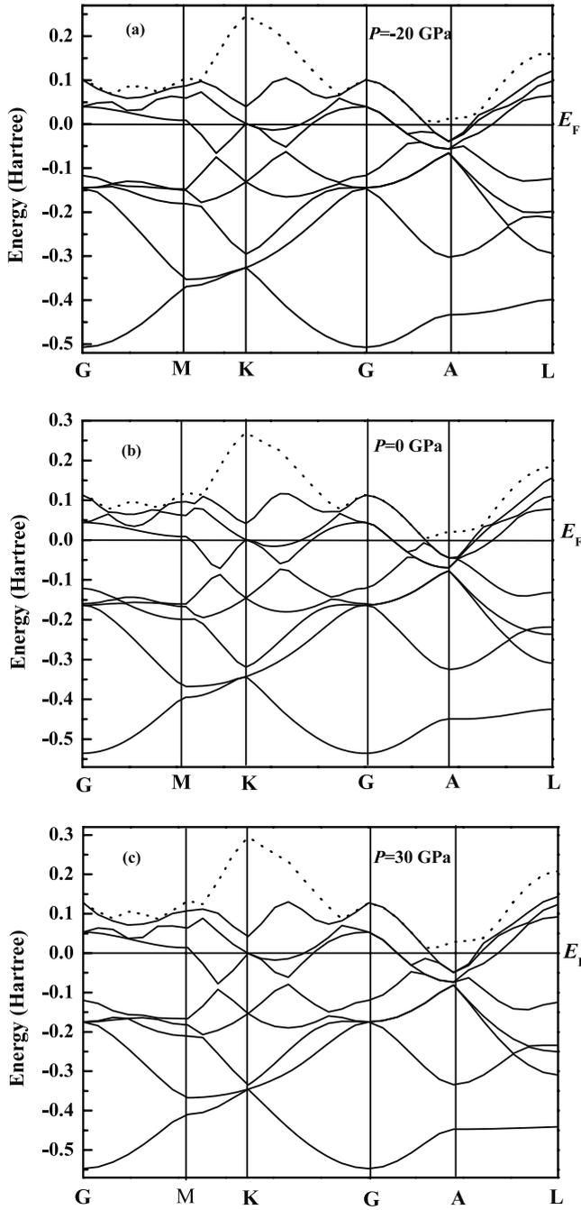
**Figure 4.** Band structure of NbB<sub>2</sub> at pressure (a) –20 GPa, (b) 0 GPa, and (c) 30 GPa, where the dotted line represents the  $\pi$  band.
