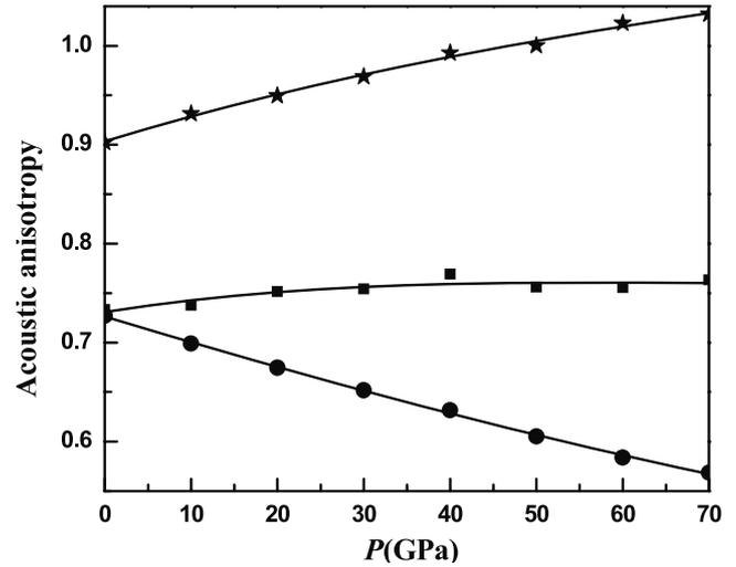
**Figure 3.** The anisotropies, elastic constant ratios  $C_{33}/C_{11}$ ,  $(C_{11} + C_{33} - 2C_{13})/4C_{44}$ ,  $2C_{44}/(C_{11} - C_{12})$ , which can determine the anisotropies of the compressional wave ( $\Delta_P$ ) and the shear wave ( $\Delta_{S1}$  and  $\Delta_{S2}$ ), are displayed as functions of various pressures. The squares, circles and stars represent  $\Delta_P$ ,  $\Delta_{S1}$  and  $\Delta_{S2}$ , respectively.
