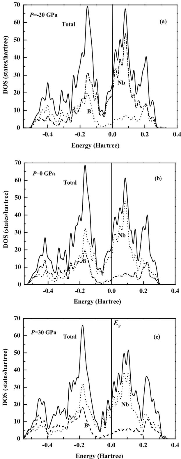
**Figure 5.** The total and partial DOS of NbB<sub>2</sub> under pressure (a) -20 GPa, (b) 0 GPa, and (c) 30 GPa.
