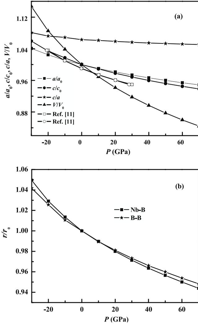
**Figure 1.** (a) The normalized volume  $V/V_0$ ,  $a/a_0$ ,  $c/c_0$ , and  $c/a$  as a function of pressure at  $T = 0$ , where the rectangles, circles, and triangles represent our obtained  $V/V_0$ ,  $a/a_0$ , and  $c/c_0$  respectively, and the blank ones are the results from [11]; (b) variation of the normalized distance  $r/r_0$  between the atoms with pressure.
