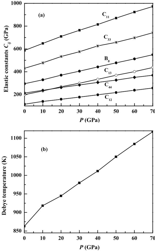
**Figure 2.** (a) The elastic constants  $C_{ij}$  and the bulk modulus  $B_0$  as a function of pressure of NbB<sub>2</sub>; (b) variations of the Debye temperature  $\Theta_D$  dependences on pressure.
