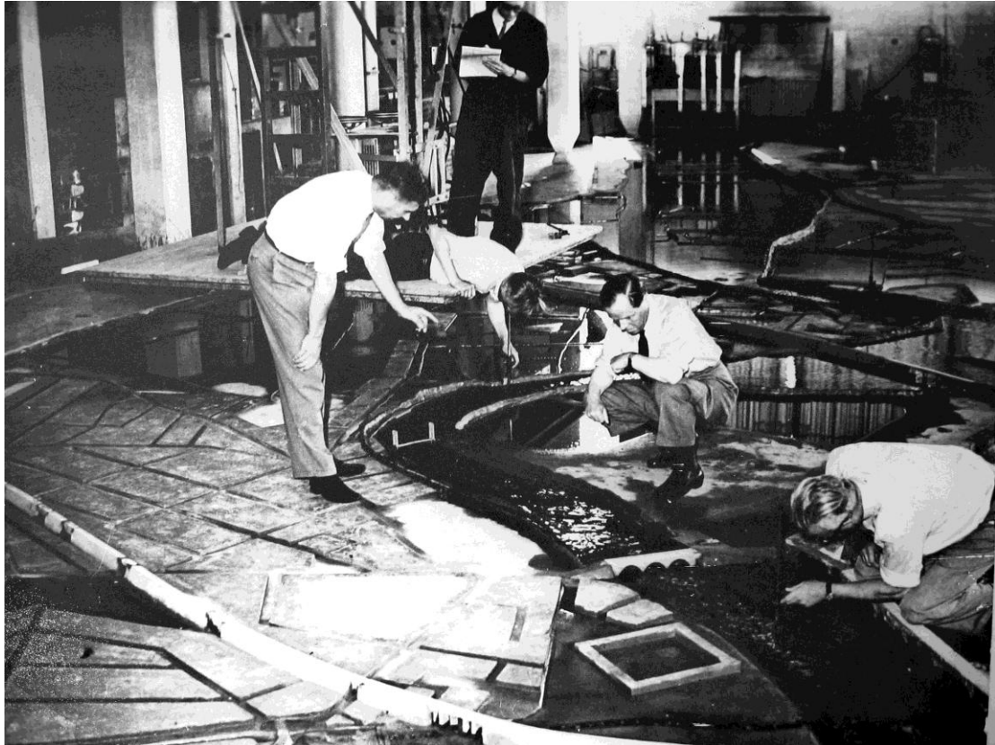
Figure 1 Study of flood countering measures using a model of the Trent river, 1947
