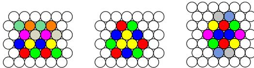
Figure 3: a) Translation of the lattice along  $\mathbf{e}_1$  ( $n = 0$ ). b) Rotation of the lattice around  $\frac{1}{3}(\mathbf{e}_1 + \mathbf{e}_2)$  through  $\pm\frac{2}{3}\pi \pmod{2\pi}$  ( $n = 2, 4$ ). c) Rotation of the lattice around  $\frac{1}{2}\mathbf{e}_1$  through  $\pm\pi \pmod{2\pi}$  ( $n = 3$ ).
