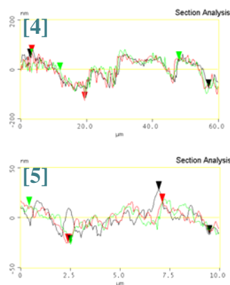
Figure 11. AFM lineouts before and after the oxidisation stage.
