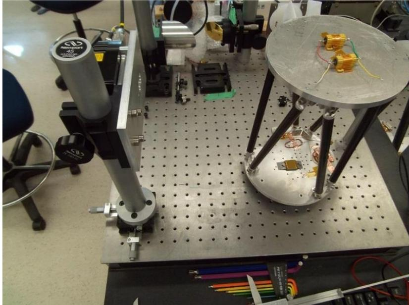
Figure 19. Testing the effect of misalignment of the mirrors in the hexapod system by scanning the laser interferometer head on an x-y translation stage.
