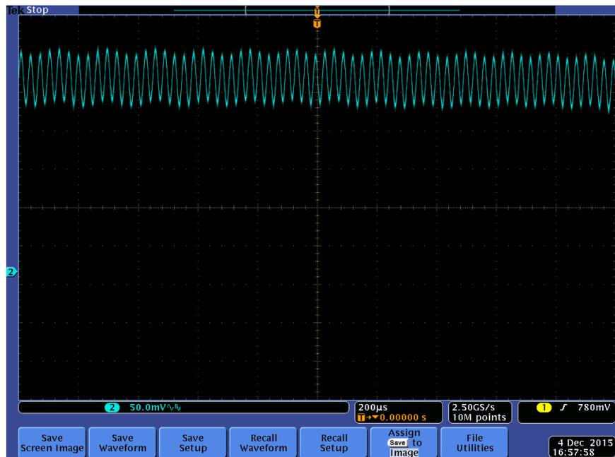
Figure 54. Interference fringes observed with a HeNe laser through the Mylar beamsplitter in the wishbone FTS. The scanning frequency of the FTS was 2 Hz.
