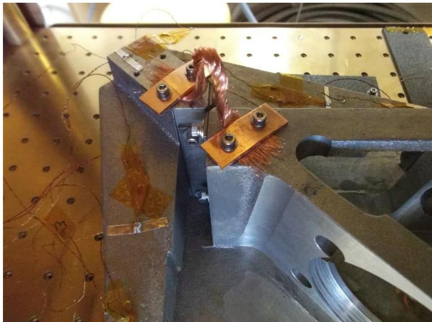
Figure 49. Flexible copper braid attached to pivot of the wishbone arm to aid cooling the arm.
