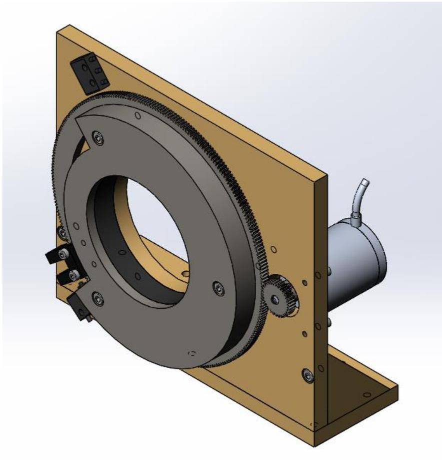
Figure 33. Design of the cryogenic iris.
