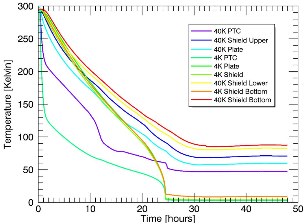
Figure 14. Temperature logs for cool down of the empty Test Facility Cryostat without precooling.
