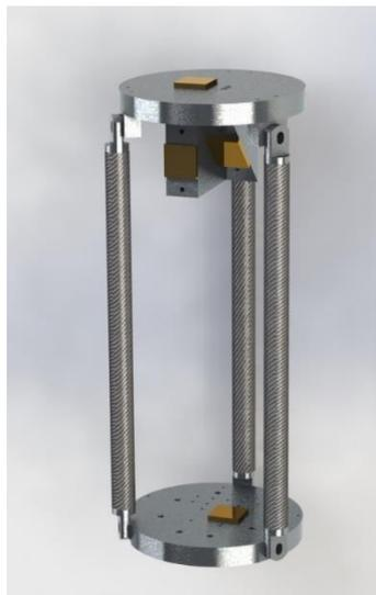
**Figure 27.** The design concept of the CFRP tripod designed to replace the hexapod. This design allows for both folded and on-axis measurement with the laser interferometer, to directly determine the thermal contraction of the CFRP struts.
