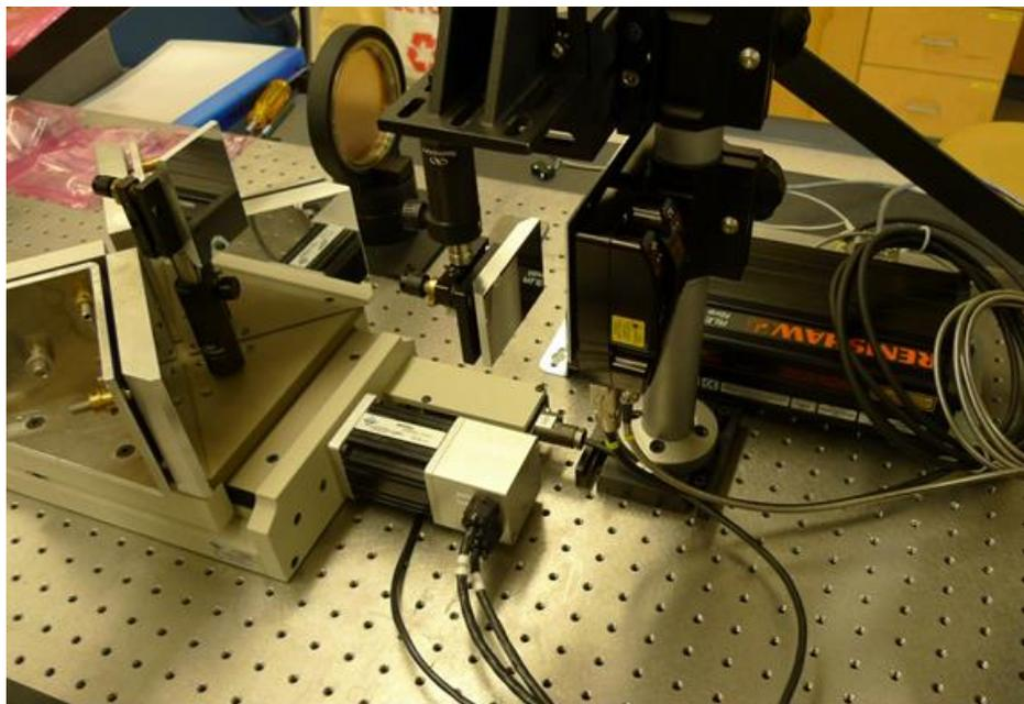
**Figure 16. Testing the laser interferometer against a Heidenhain linear encoder. The interferometer head is shown at the centre mounted to the vertical post. The stationary reference mirror can be seen to the left of the head; the moving mirror is mounted at the apex of the FTS moving mirror assembly at the left.**
