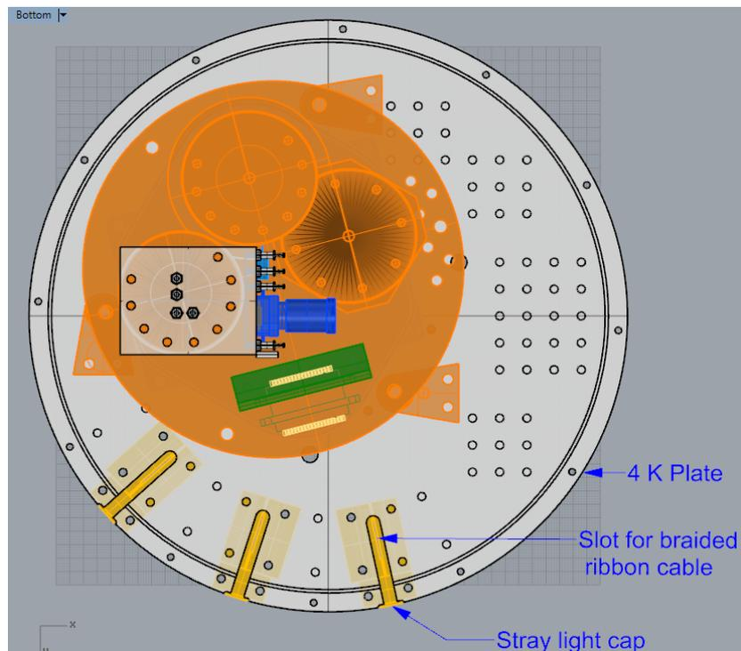
Figure 8. Slots in 4 K plate for heat sinking the wiring whereas 77 K plate has the similar slots and heat sinking plates.
