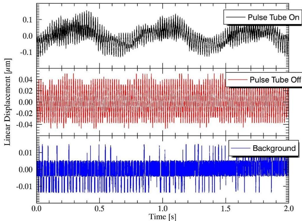
Figure 23. Noise measurement time series from the Renishaw DI: a) Normal operation; b) Pulse tube off, vacuum pump on; c) Background noise (everything off).
