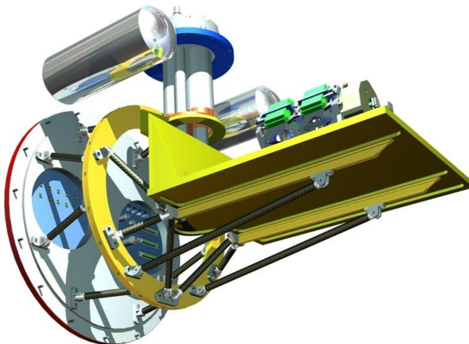
**Figure 10. Internal components of the original cryostat design, with horizontal 4 K work surface supported by cantilevered CFRP struts and cooled by a single PT415 pulse tube cooler.**
