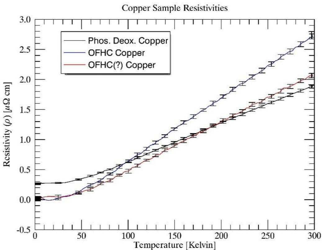
Figure 34. Measured resistivity as a function of temperature for various copper samples.
