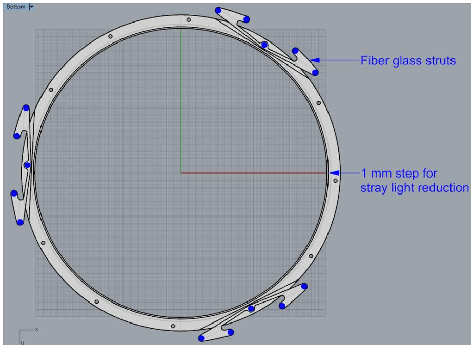
Figure 5. Mating flange between the two 4 K shields.
