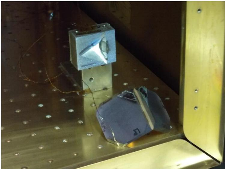
**Figure 44.** The original corner cube retroreflectors from the WBI after thermal cycling. The dislocation is due to the differential thermal expansion of the aluminum frame and the glass mirror.
