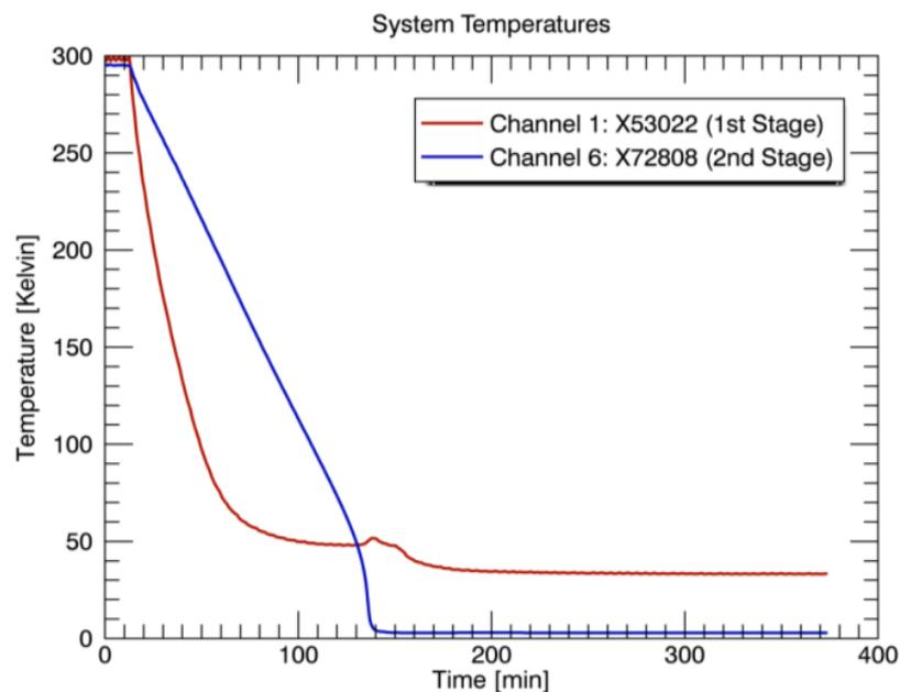
Figure 3. Typical temperatures of the pulse tube cold heads during a cool down of the empty cryostat.
