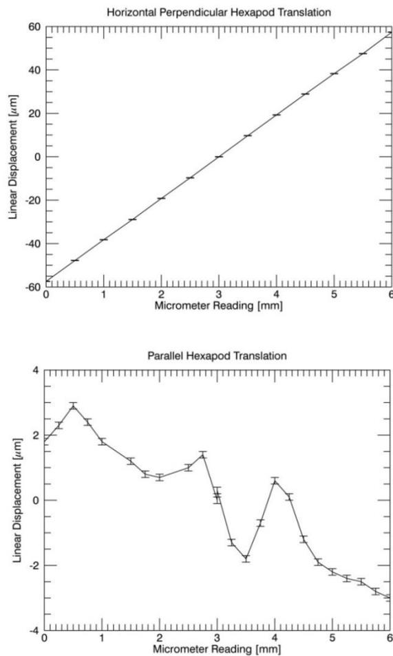
Figure 20. Measurement error due to motion of the interferometer head perpendicular to the beams (top) and parallel to the beams (bottom). The differential measurement effectively cancels parallel motion, but is sensitive to drift of the beams across the tilted mirrors.
