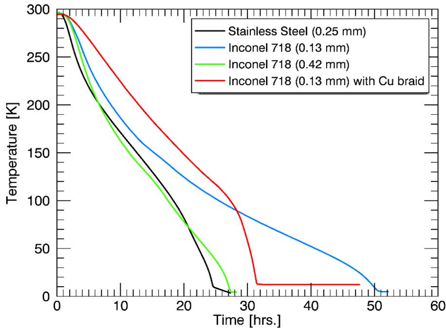
Figure 48. Temperature of the WBI arm during cooling. Nominal cooling time for the 4 K volume is 23 hours.
