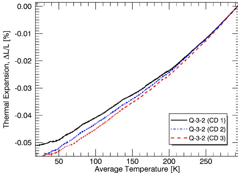
Figure 32. Variation in thermal expansion over three cooldown cycles for a single set of samples.
