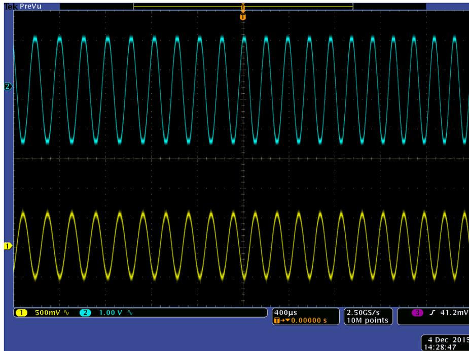
Figure 52. Oscilloscope readout of the IR metrology fringes while scanning the mirror at nearly constant velocity.
