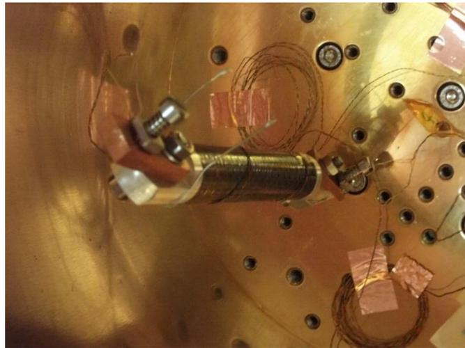
Figure 24. CFRP strut mounted on the 4 K for thermal conductivity measurements.
