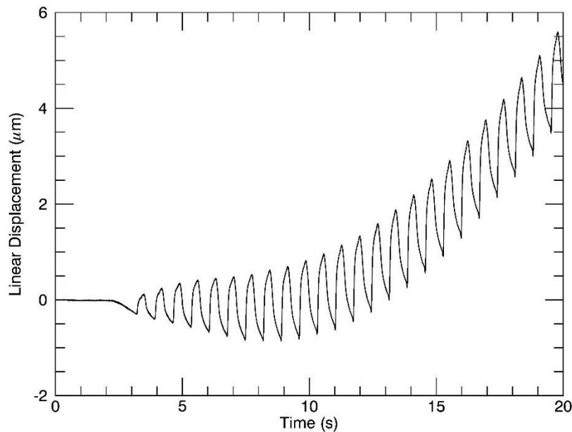
**Figure 21. Measured displacement in the hexapod structure as the pulse tube cooler is turned on. The ~1 Hz oscillations are due to pressure waves in the pulse tube; the slow drift is due to contraction of the hexapod and cryostat structures.**
