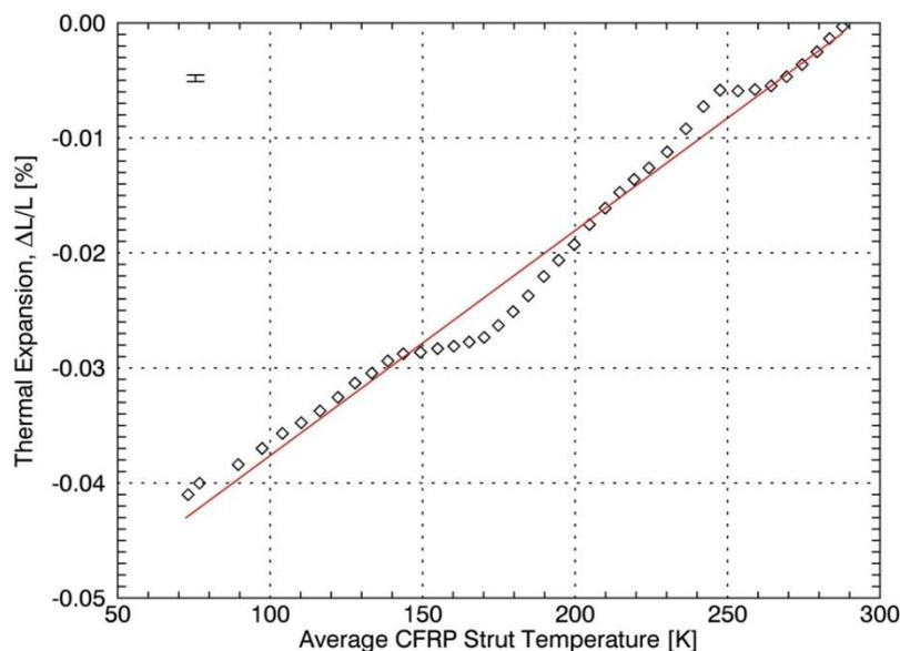
**Figure 28. Temperature dependent thermal expansion of CFRP struts in the tripod assembly. Data points were fit with a 1<sup>st</sup> order polynomial to determine average CTE.**
