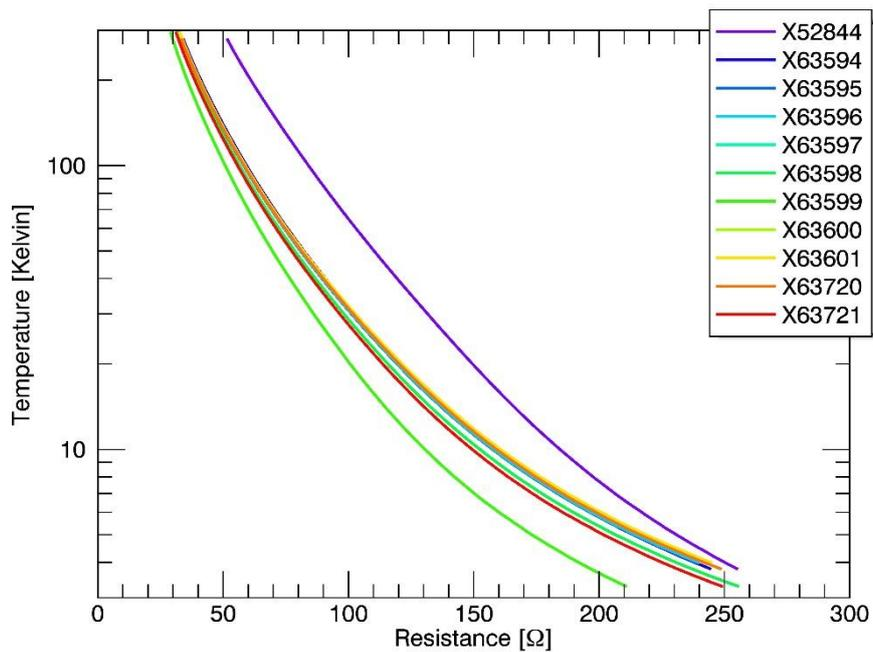
Figure 2. T(R) calibration curves generated in the lab for 11 CX-1010-SD resistance temperature detectors.
