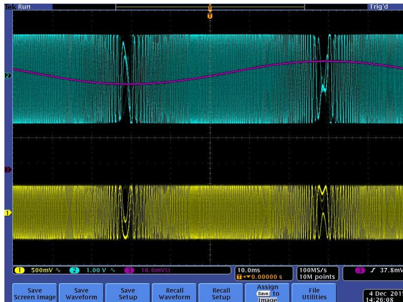
Figure 51. Oscilloscope readout of the frequency modulation in the IR metrology fringes due to the sinusoidal velocity of the mirror.
