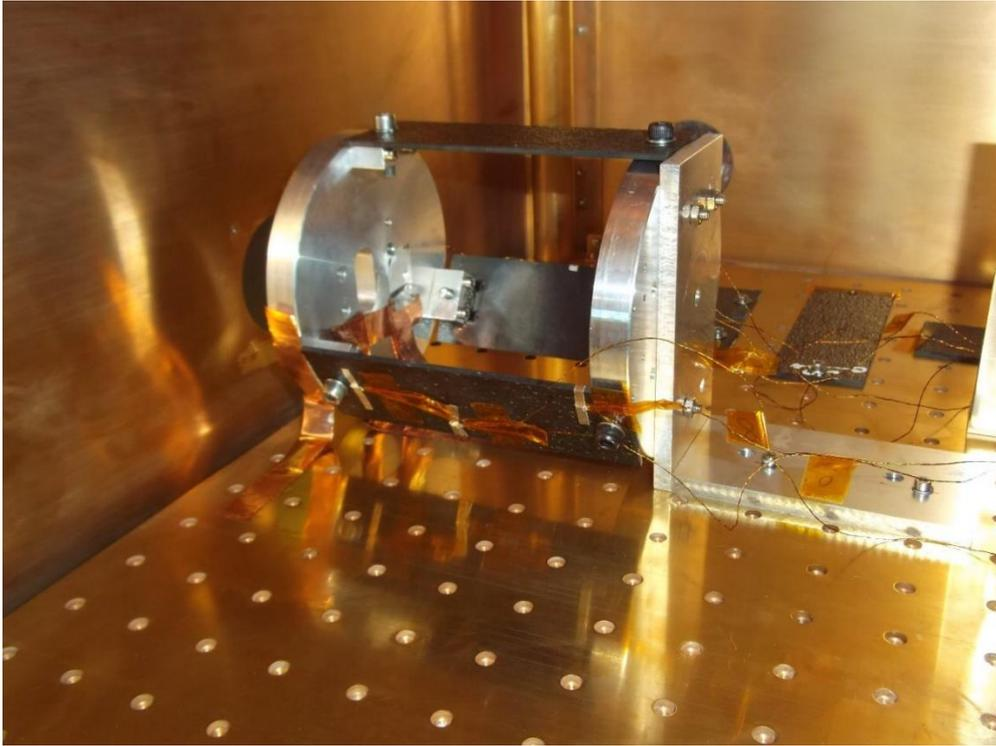
Figure 30. CFRP contraction measurement jig installed on the TFC 4 K plate. The beams from the Renishaw Differential Interferometer enter through the cryostat window on the left.
