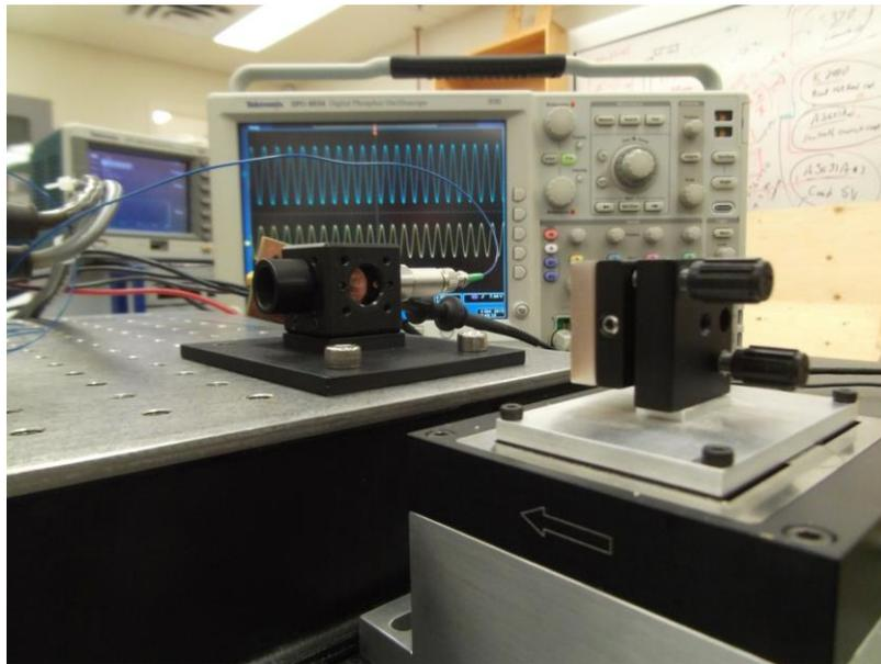
Figure 50. IR metrology system shown on an optical bench for testing. Fringes on the oscilloscope are the result of modulating the path difference by translating a reflecting mirror.
