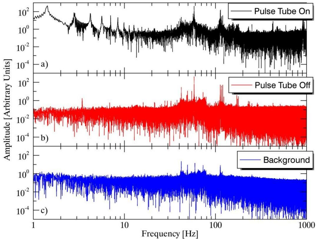
**Figure 22. Power spectrum of displacement noise measured with the Renishaw DI: a) Normal operation; b) Pulse tube off, turbo vacuum pump on; c) Background noise (cooler and pump off).**
