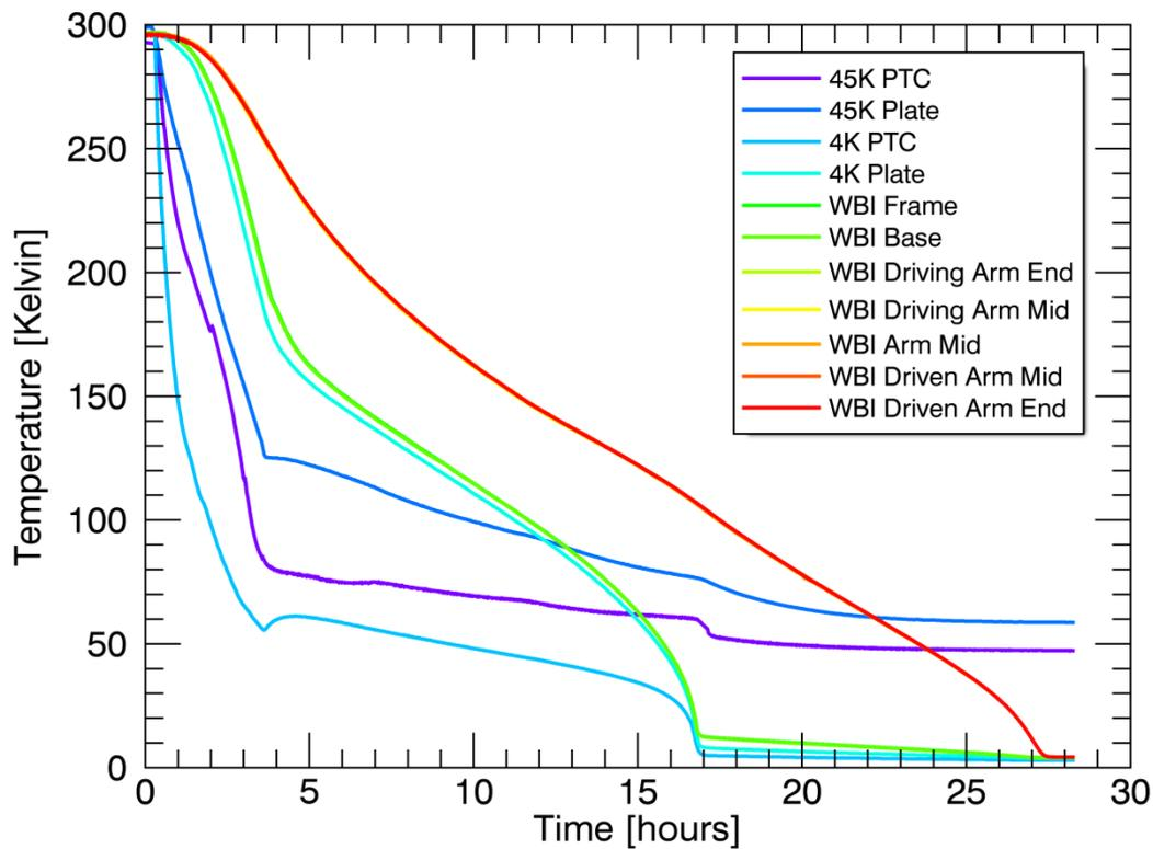
Figure 47 Thermal map of the wishbone interferometer
