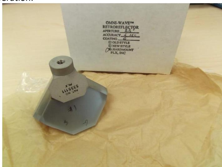
**Figure 45.** Replacement corner cube retroreflectors with Invar frame. These corner cubes were tested at 4 K and maintained alignment both while cold and on return to room temperature.
