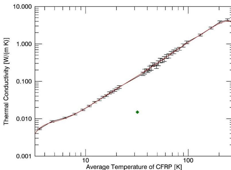
Figure 25 Measured thermal conductivity as a function of temperature for the CFRP strut, with measurement errors. The single green diamond indicates the single conductivity value determined in previous measurements. The red line indicates the polynomial fit to the data. The gap between 20 and 40 K was due to a computer malfunction during the cool down.
