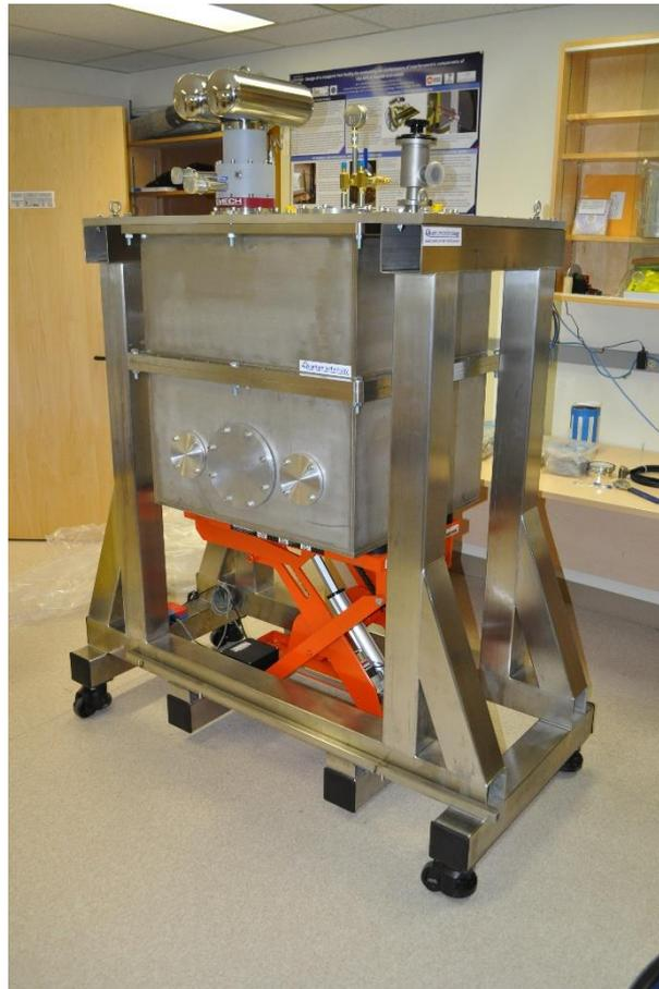
**Figure 12. Outer vacuum chamber for the test facility cryostat, showing one of the large aperture viewports and two smaller 50mm diameter ports. These viewports are mirrored on the rear side, and three additional 50 mm diameter ports are located on the short sides and bottom of the vacuum chamber for the Renishaw differential interferometer.**
