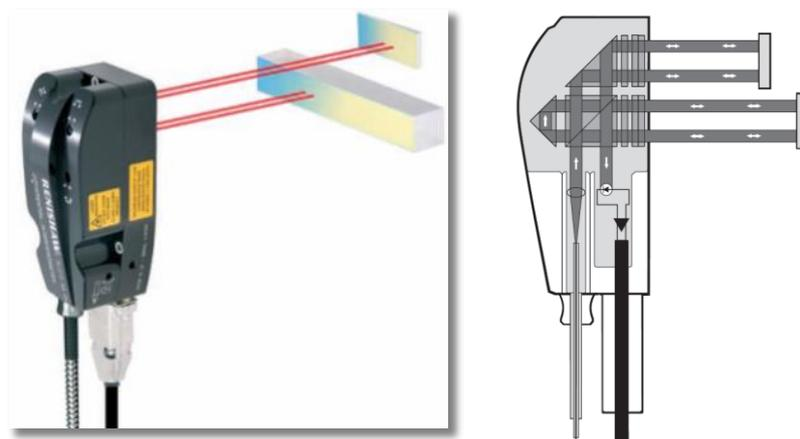
**Figure 15. Renishaw Differential Laser Interferometer uses two pairs of optical laser beams to measure the relative displacement between two plane mirror targets. A quadrature signal is produced, indicating relative displacement magnitude and direction.**
