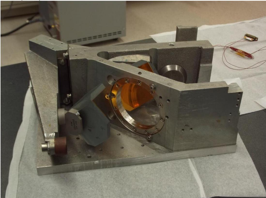
Figure 53. Image of the wishbone interferometer with a Mylar beamsplitter.
