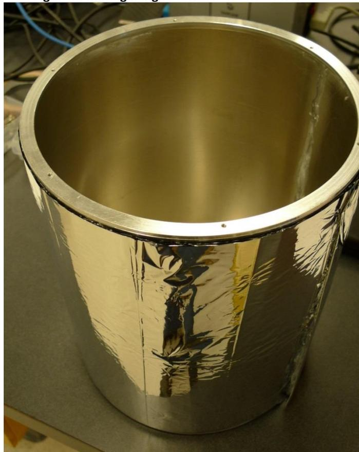
Figure 6. One section of the 77 K shield with MLI blanket.
