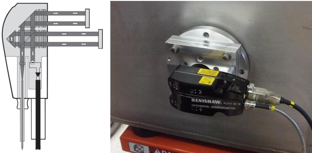
Figure 29. Schematic of the Renishaw Differential Interferometer and mounting plate for the TFC
