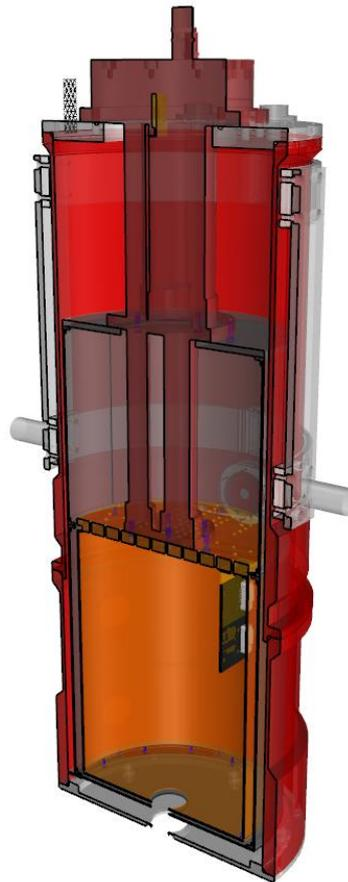
Figure 1 (left) Assembled cryostat with vacuum vessel removed showing upgraded 77 K shield and superinsulation. (right) Cross-section rendering showing inverted system with upgraded 4 K and 77 K shields and bottom-viewing window.
