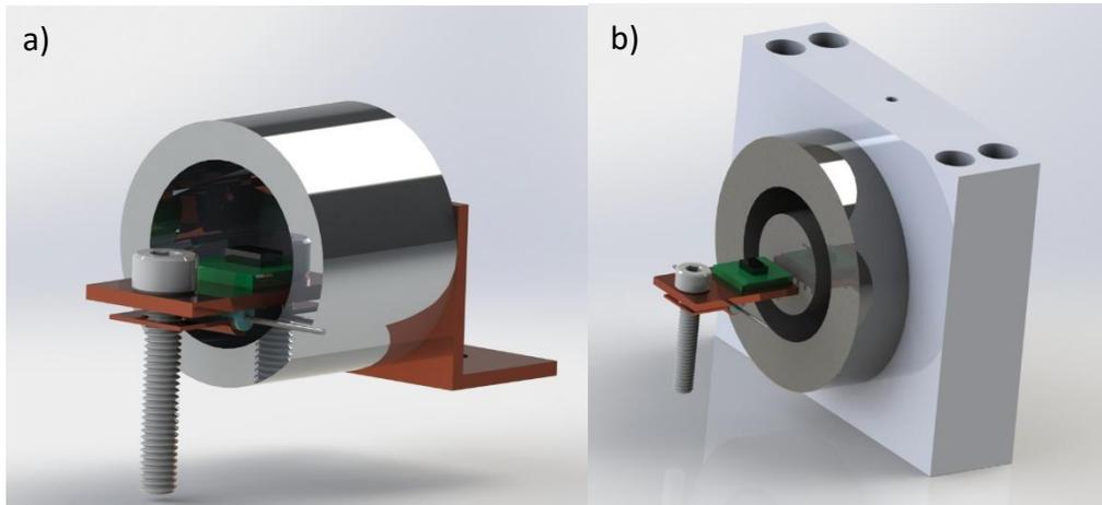
Figure 39. Setup for measuring the 4 K performance of Hall effect sensors within: a) the solenoid and b) the voice coil magnet.
