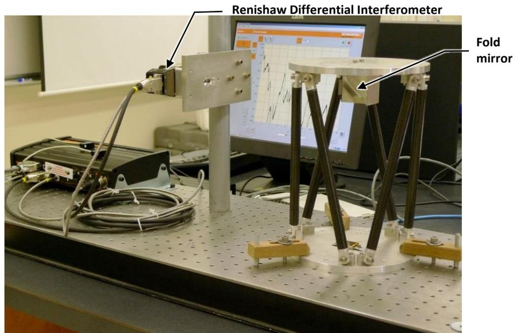
Figure 18. Testing the hexapod design concept on the bench. The diagonal fold mirror is shown hanging off the top plate of the hexapod.
