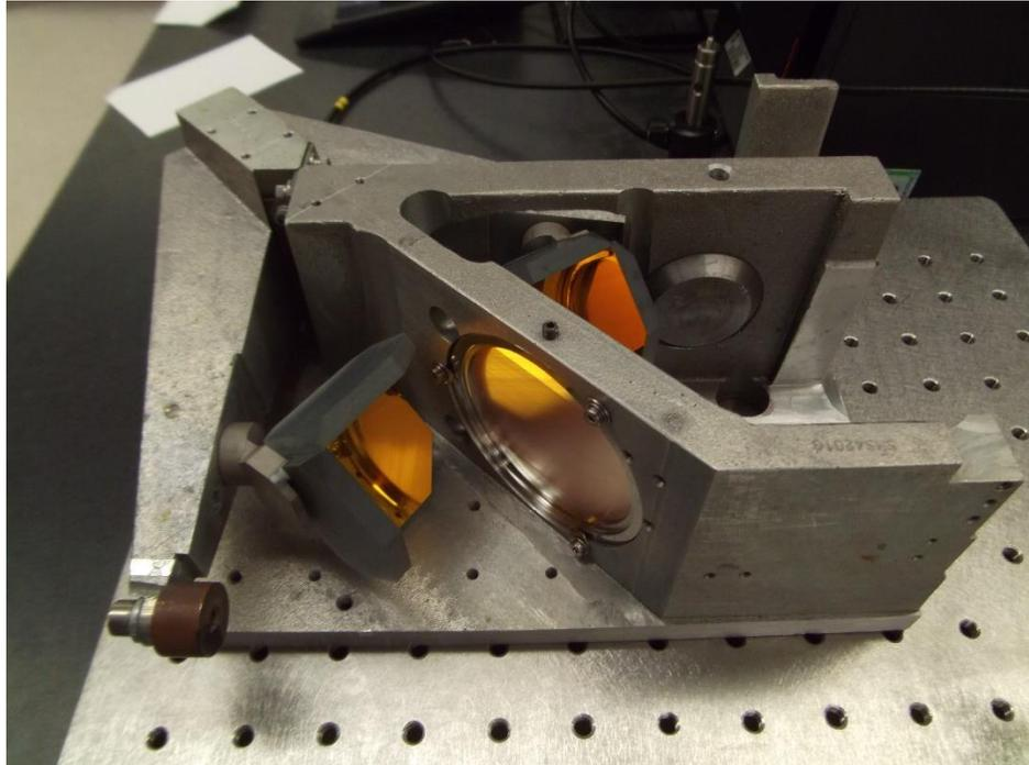
Figure 37. The ABB FTS mechanism retrofitted with thermally stable mirrors and far-IR beamsplitter.
