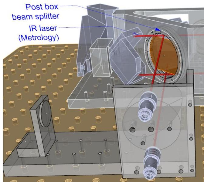
Figure 43. Sheared metrology beams in the interferometer, passing through the custom beamsplitter.
