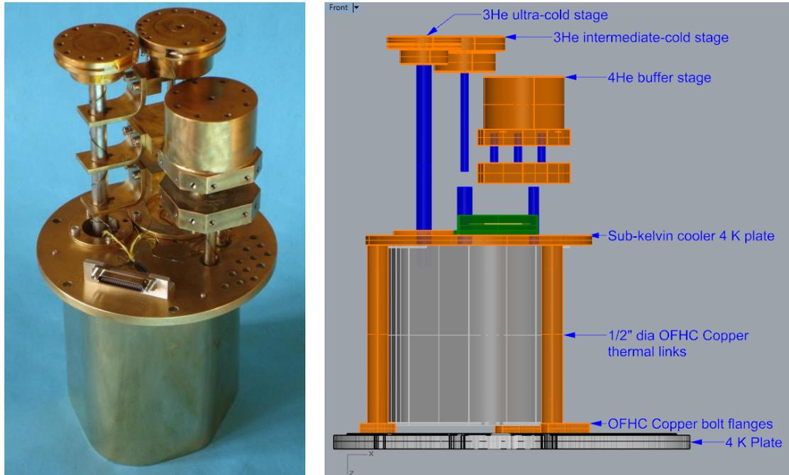
Figure 4  $^3\text{He}$ - $^4\text{He}$  fridge (left). Thermal links between fridge and 4 K plate (right).
