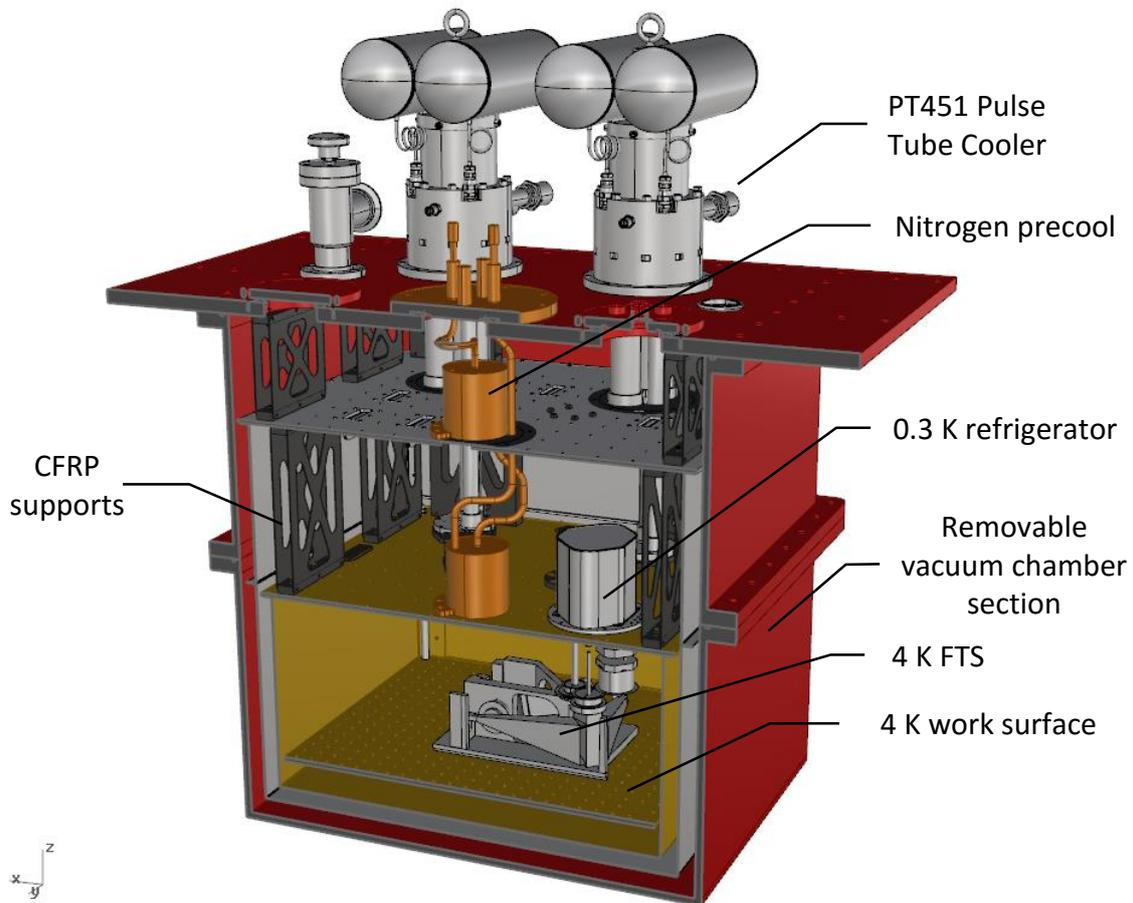
**Figure 11. Cutaway view of the large test facility cryostat final design.**
