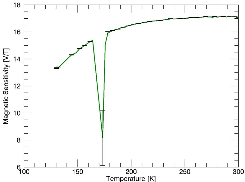
Figure 40. Temperature dependence and minimum operating temperature of the InfineonHall Current sensor with integrated amplifier electronics.
