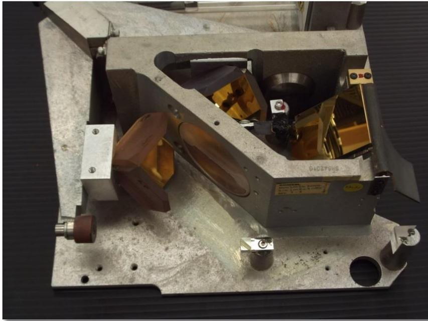
Figure 35. The ABB interferometer, with wishbone mechanism, original dual corner-cube retro-reflectors, and original IR beamsplitter.
