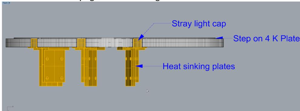
Figure 9. 4 K plate showing the copper heat sink clamps for up to 3 pairs of ribbon cables, and stray light caps.
