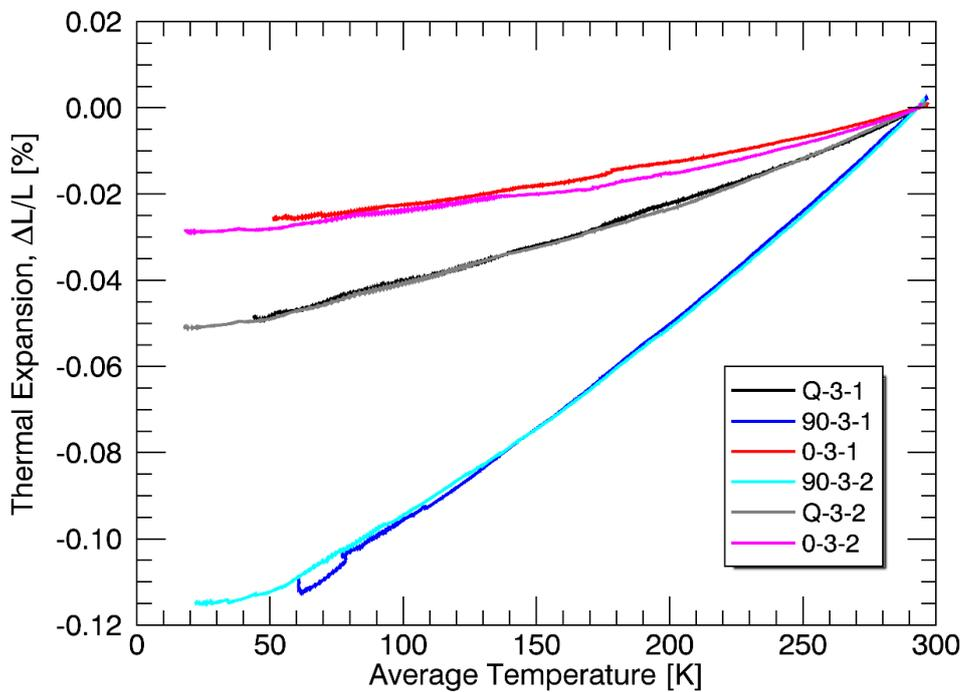
Figure 31. Thermal expansion of the Glyndwyr CFRP plate samples. The plates of each material type were cut from single sheets from the manufacturer.
