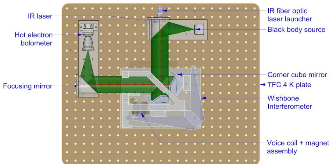
Figure 38. Schematic of the planned optical layout for the cryogenic Michelson FTS on the 4 K plate, including the ABB scan mechanism, two off-axis parabolic reflectors, low temperature blackbody source, 0.3 K detector and feedhorn.
