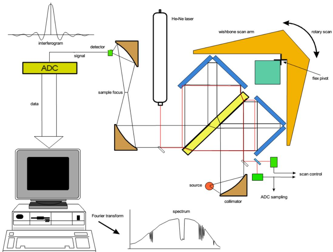
Figure 36. Schematic showing the ABB interferometer optics as well as the measurement and metrology beams.
