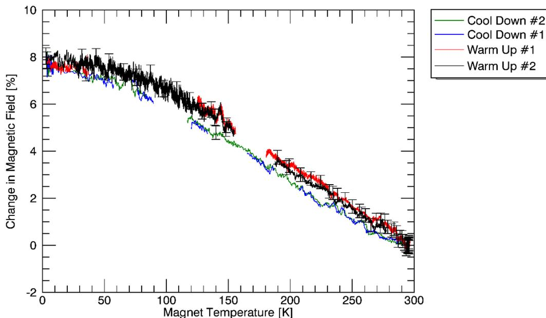
Figure 41. Percentage change in the magnetic field strength of the permanent magnet of the WBI voice coil. Measurements were taken over two complete thermal cycles of the magnet to 4K. Offset between the cool down and the warm up curves demonstrates a small amount of hysteresis upon thermal cycling. All magnetic field strength changes are reversible.
