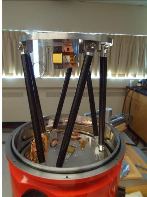
**Figure 26.** The CFRP hexapod mounted inside the cryostat. A mirror block is attached on the underside of the upper plate with a vertical mirror for the reference beam of the interferometer and a tilted mirror that deflects the measurement beam to the mirror on the 4 K work surface.
