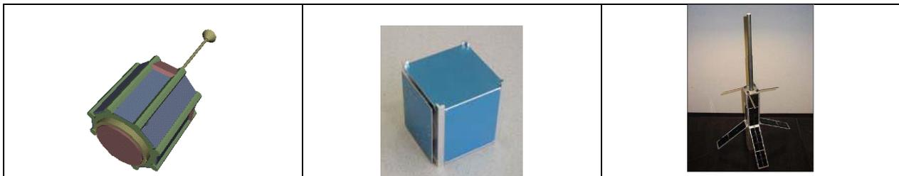
**Figure\_6.1.1-1** - LEFT: 3D view of WebSat: a nanosatellite broadcasting Earth pictures on-line in real time. MIDDLE: Picture of CUTE-1, a 1U cubesat developed to tests commercial components. RIGHT: Picture of Quake Sat, a 3U cubesat developed to detect low frequency emissions during earthquakes.
