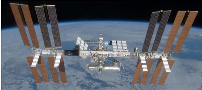
**Figure\_3.2.3-33.** *The international space station, built around a 109m long truss.*
