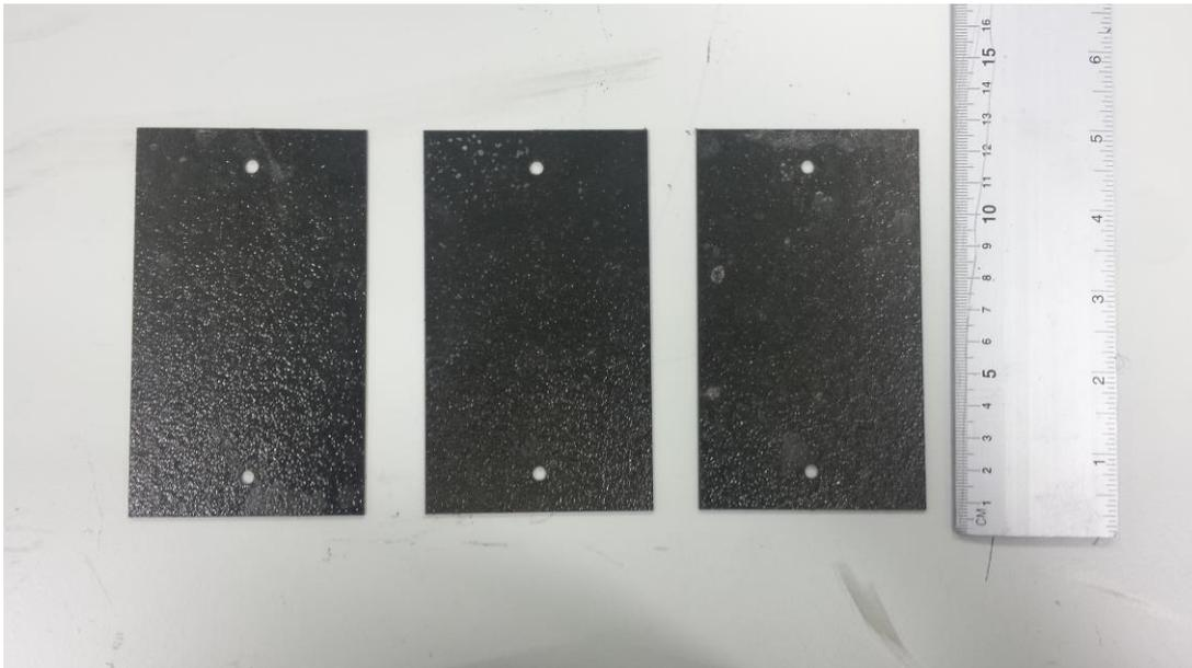
**Figure 5: CFRP samples for cryogenic testing**
