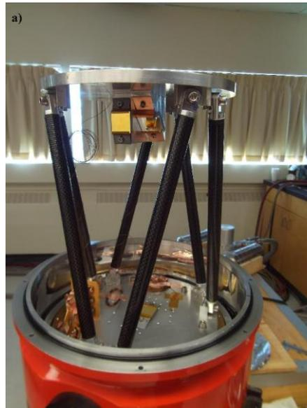
**Figure 4: Hexapod structure for 6L 4K cryostat**
