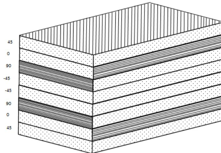
**Figure 3: Ply stacking sequence of a laminate**
