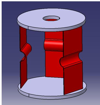
**Figure 6: CAD mock-up of ILSS test**
