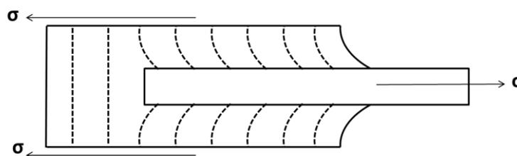
Figure 2: Resin deformation pattern when fibre is subjected to a tensile load
