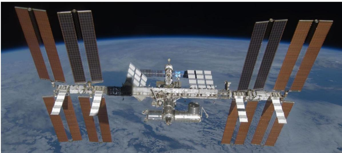
*Figure 10. The international space station, built around a 109m long truss.*
