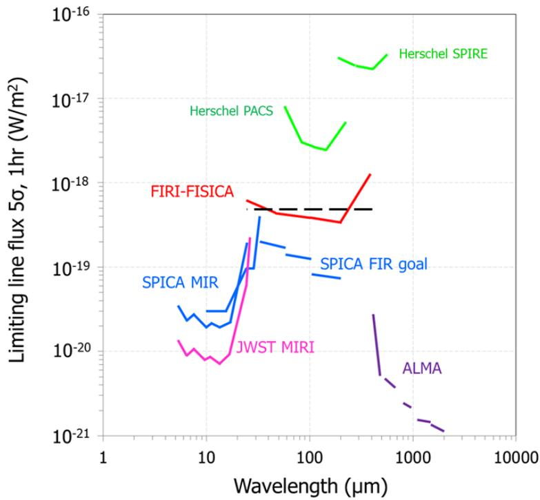
**Figure A1:** (Top) Point-source detection limit ( $5\sigma$ , 1hr) for spectrophotometry ( $R=5$ ) for FIRI-FISICA and other missions; (Bottom) The limiting line flux achievable from a point-source ( $5\sigma$ , 1hr) for FIRI-FISICA and other missions. The dashed black lines give the approximate sensitivity requirements levels as outlined in this document (section 2.4) in each case.
