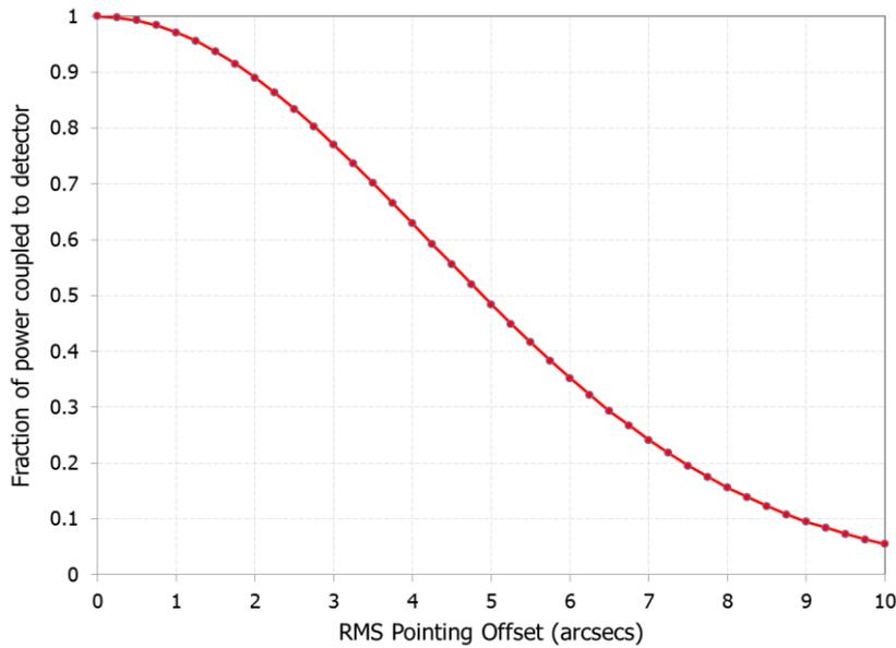
**Figure 4:** The coupling efficiency to a point-source as a function of RMS telescope pointing error.
