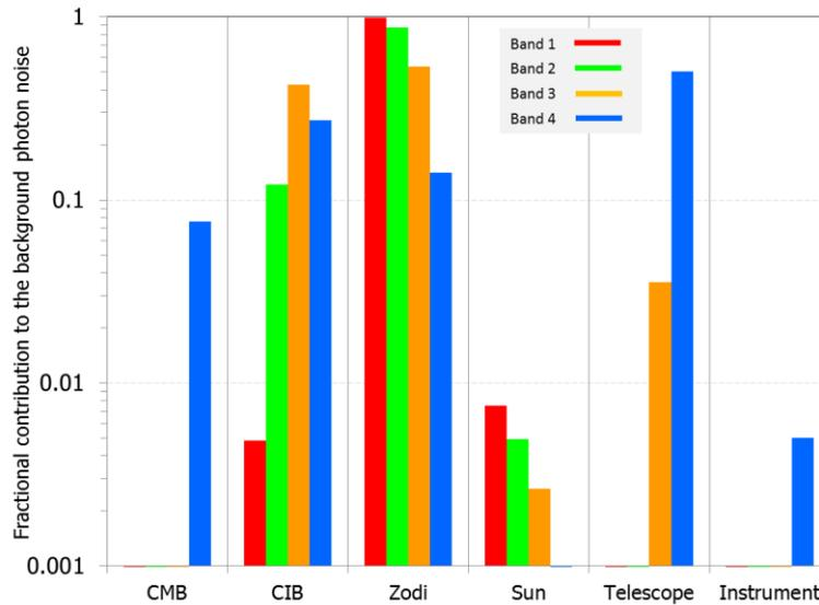
**Figure A1.1:** The relative contribution to the overall photon noise from the sky, telescope and instrument for the 4 wavebands.
