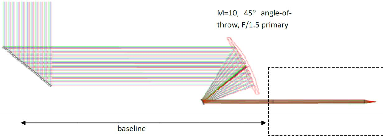
Figure 2: Optical configuration for the “BETTII-type” design.
