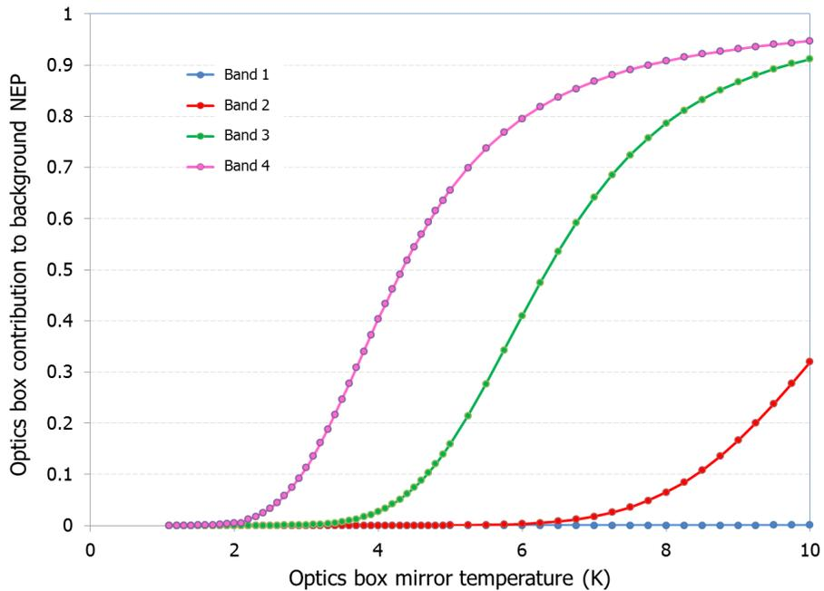
**Figure 6:** The contribution of photon noise from the optics box mirrors as a fractional of the overall background NEP as a function of mirror temperature. This assumes the telescope mirrors are operating at 4.5K.
