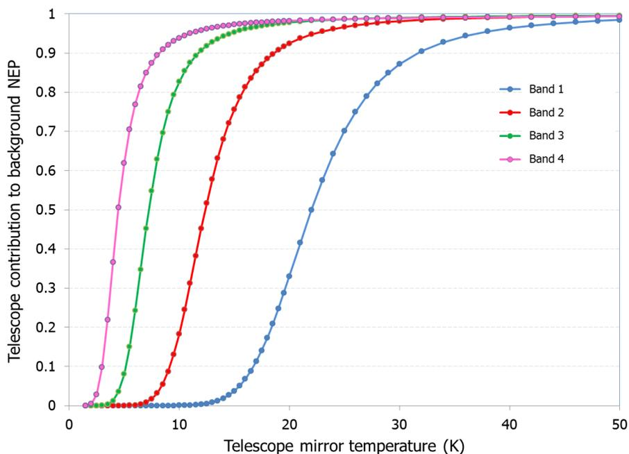
**Figure 3:** The contribution of photon noise from the telescope as a fractional of the overall background NEP as a function of telescope temperature. This assumes any subsequent optics has a negligible contribution to the background.
