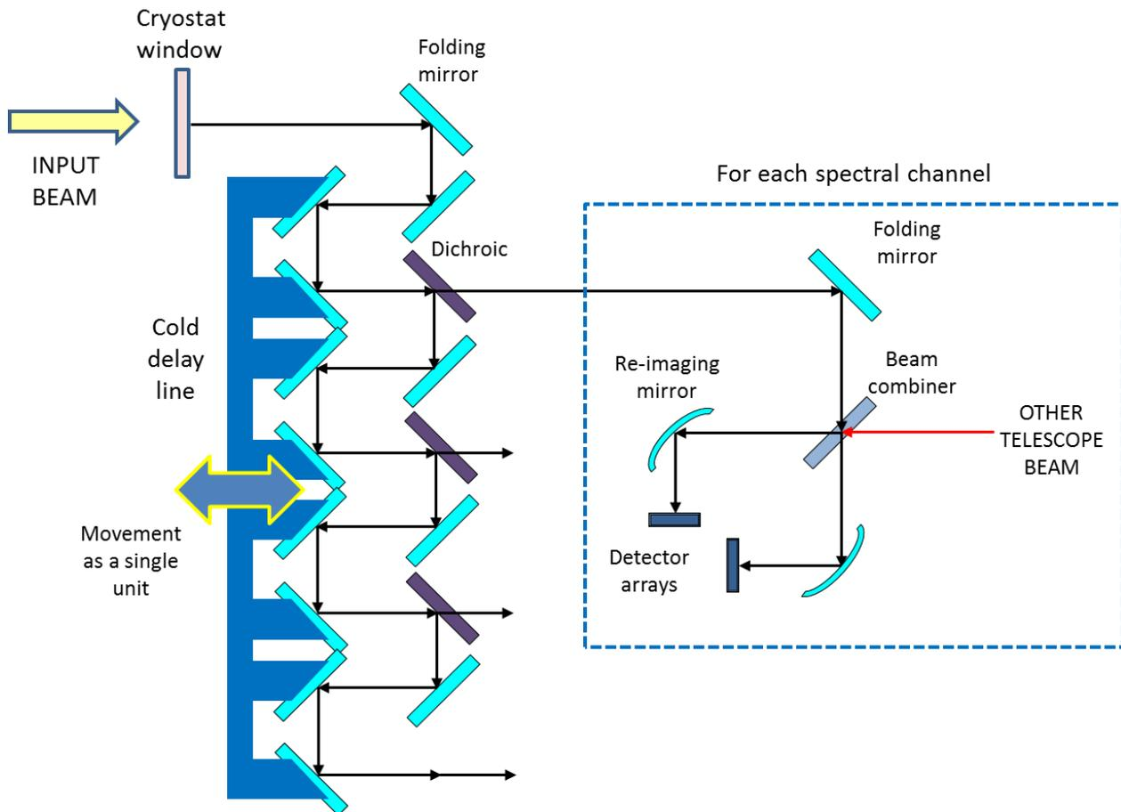
Figure 5: A schematic representation for the possible layout of the instrument cryostat.
