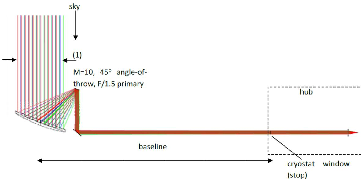
**Figure 1:** Optical configuration for the "FIRI-type" design.
