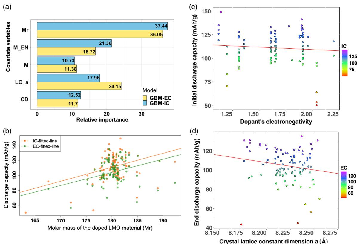
**Figure 4.** a) The relative importance of the model input variable for the prediction of the initial (IC) and the 20th cycle end discharge capacity (EC) estimated by the optimized GBMs. b) The plot of the values of IC and EC against the molar mass of the doped LMO cathode material with the linearity fitted lines for the whole dataset. c) The plot of IC against dopant's electronegativity with the red best-fitted line. d) EC versus crystal lattice constant-*a* with the red best-fitted line.
