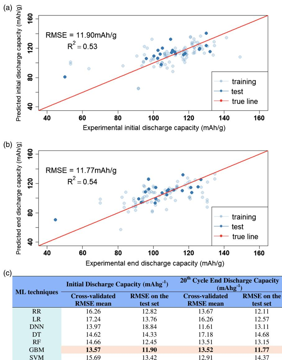
**Figure 3.** a) Scatter plots of experimental values against the predicted value for initial capacity and b) 20th cycle end capacity performed by the GBM. c) The mean RMSE values for during the tenfold cross-validation and for testing against 20 holdout test dataset for the prediction of Initial discharge capacity and end discharge capacity.
