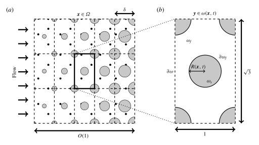
FIGURE 1. Model schematic in two dimensions. (a) An example in which the macroscale porosity decreases in the direction of the flow. (b) A magnified view of a given cell  $\omega(\mathbf{x}, t)$ , with microscale coordinate  $\mathbf{y} \in [-1/2, 1/2] \times [-\sqrt{3}/2, \sqrt{3}/2]$ .
