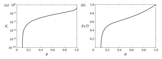
FIGURE 2. The functions (a)  $\mathcal{K}(\phi)$  and (b)  $Pe\mathcal{D}(\phi)$  (defined in (3.8b) and (3.18b), respectively) calculated using Comsol Multiphysics, for circular obstacles whose centres lie on a hexagonal lattice.
