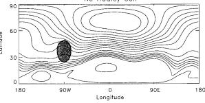
Fig. 12. Contour plots showing the time mean PV fields in the longtime  $\epsilon=0.5$  isolated mountain experiments. The contour intervals are  $0.2~\Omega H^{-1}$ .
