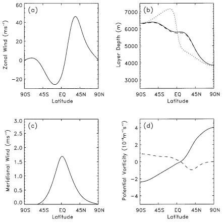
FIG. 1. The shallow-water basic-state circulations used in the experiments. (a) Zonal mean zonal wind  $u_0^H (=u_0^N)$ . (b) Zonal mean thickness  $\sigma_0^H$  (solid curve),  $\sigma_0^N$  (dashed curve), and radiative equilibrium height  $\sigma^{eq}$  (dotted curve). (c) Meridional wind  $v_0^H$ . (d) Potential vorticity  $P_0^H$  (solid curve) and  $(P_0^H - P_0^N) \times 100$  (dashed curve).
