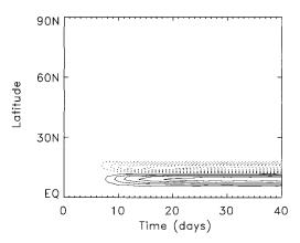
FIG. 5. Contour plot showing the difference in the evolution in latitude and time of  $\nabla \cdot \overline{\mathbf{F}}$  between the two linear experiments. The sense is  $\langle \text{Hadley circulation case} \rangle - \langle \text{no-Hadley circulation case} \rangle$ . The contour interval is  $0.002~\epsilon^2 H\Omega^2 a$ ; positive contours are solid; and negative contours dotted. The zero contour is omitted.
