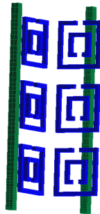
Figure 4: Configuration of the unit cell of DNM-1 consisting of metallic split ring resonators and wires as described in [21]
