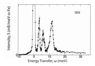
**FIGURE 3.** The scattered intensity at 10 K, averaged over  $q = 2 \pm 0.13$  Å<sup>-1</sup>, for incident energies of 10, 25, and 50 meV.
