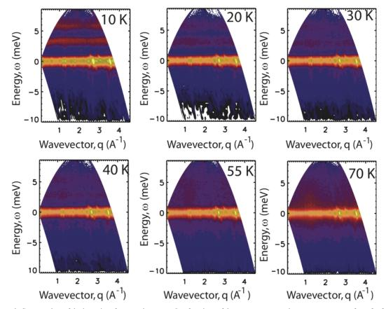
**FIGURE 2.** Contour plots of the intensity of scattered neutrons S as functions of the wave vector q and neutron energy transfer  $\omega$  for fayalite at temperatures above and below the 65 K Neel temperature. In each case, the incident neutron energy was 10 meV.
