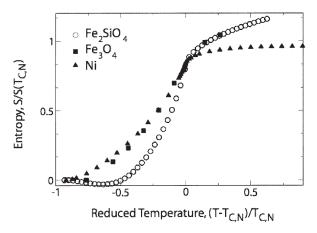
**FIGURE 10.** The evolution of the magnetic entropy in fayalite (this work), magnetite (Gronvold and Sveen 1974), and nickel (Meschter et al. 1981) with the temperature scaled to the magnetic ordering temperature ( $T_{CN}$ ), and the entropy scaled to the value at the ordering temperature.
