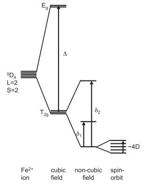
**FIGURE 7.** The subsequent effects of a cubic crystal field, a non-cubic field, and the spin orbit coupling on the states of the  $Fe^{2+}$  ion.
