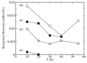
FIGURE 5. Dependence of integrated inelastic peak intensities on temperature at a fixed wavevector of  $2 \pm 0.25$  Å<sup>-1</sup> as determined from Gaussian fits to the peaks.
