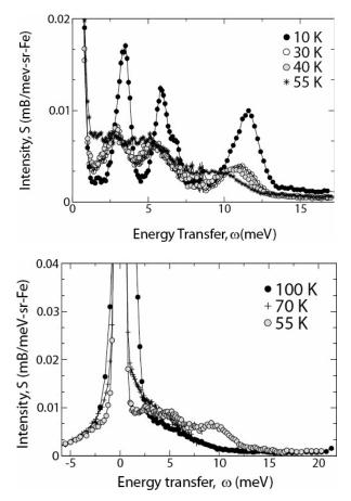
FIGURE 4. Dependence of the scattering on temperature for a fixed wave vector of  $2 \pm 0.25$  Å<sup>-1</sup>: (a) spectra from 10–55 K (b) spectra from 55–100 K.
